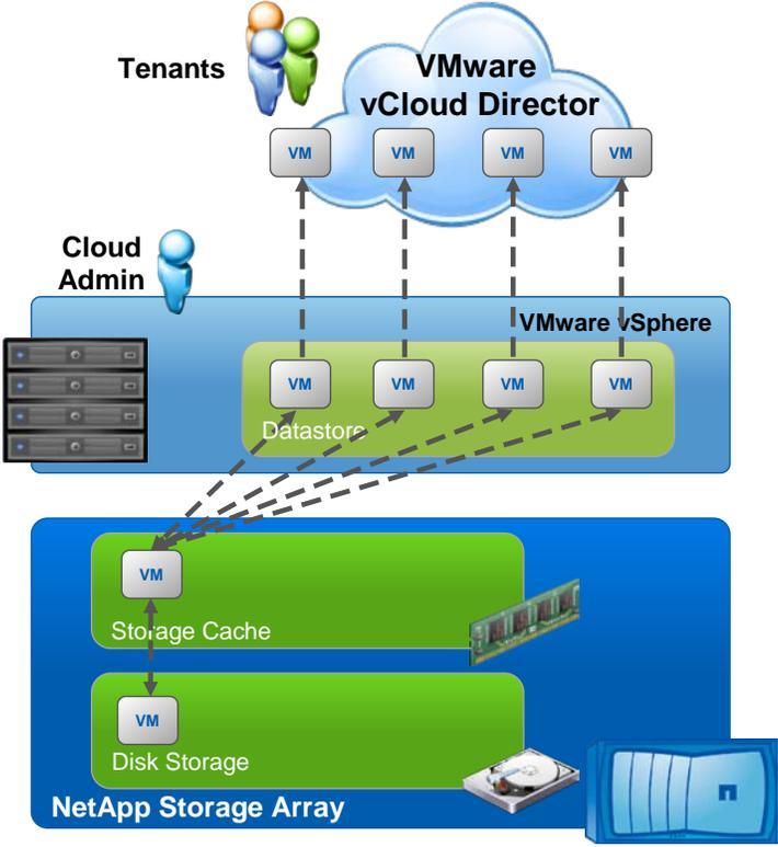
Figure 2) VM Provisioning and storage consumption on NetApp storage.
