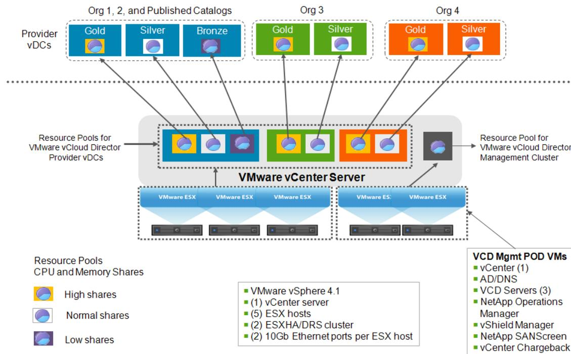
Figure 5) VMware vSphere architecture.
