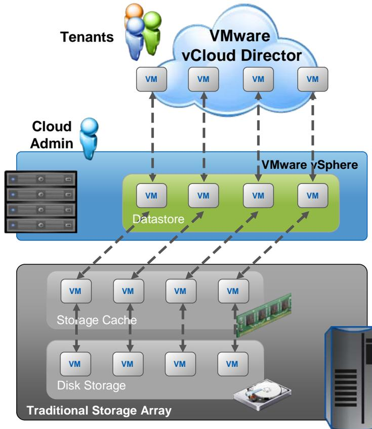
Figure 1) VM Provisioning and storage consumption on traditional storage.
