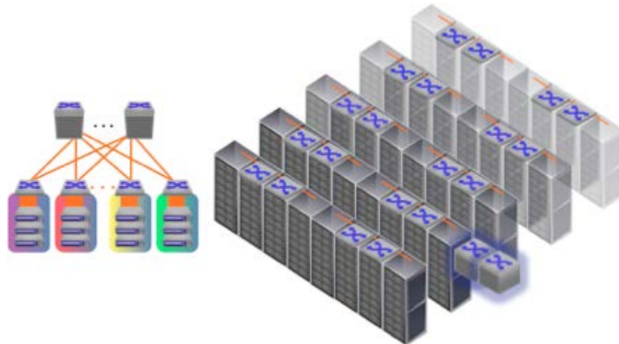
Figure 6. Two-tier Leaf-Spine Design
