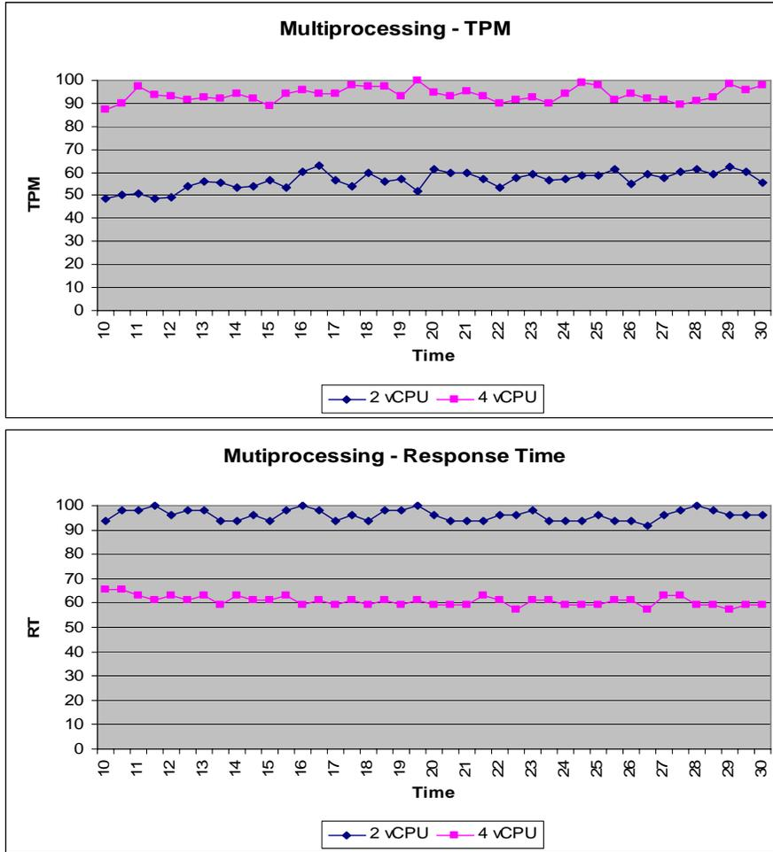
Figure 3. TPM and response time comparison between two vCPU VM and four vCPU VM
