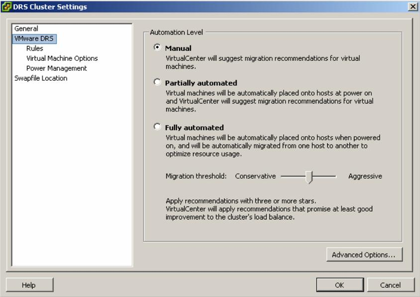
**Figure 7. VMware DRS automation level settings in a VMware ESX cluster**
