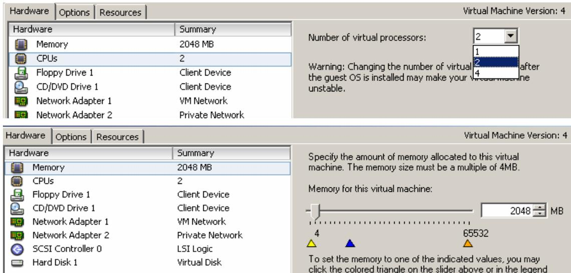
**Figure 2. Virtual CPU and memory resource change in Virtual Machine Properties**
