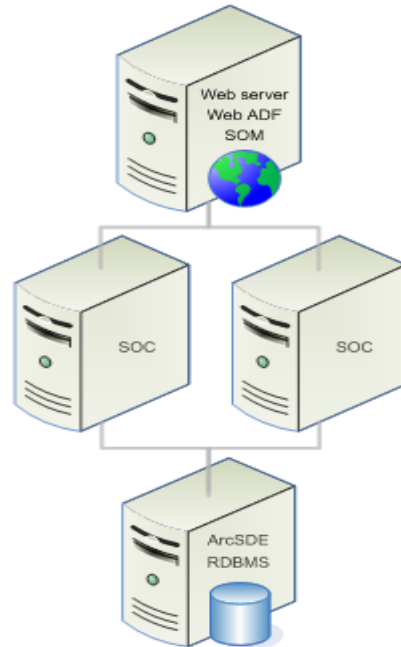
Figure 4. Multiple-Machine ArcGIS Server Deployment
