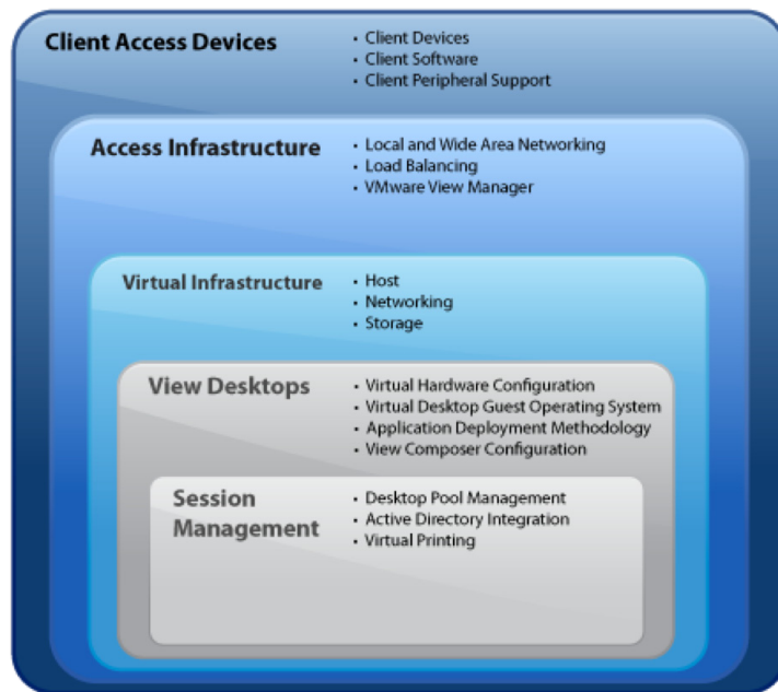
Figure 1. VMware View Component Sub-layers
