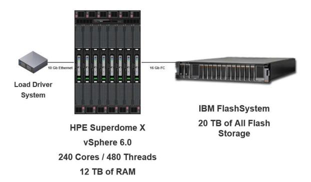
Figure 1. Testbed hardware
