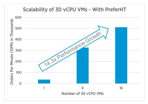
This large number of monster VMs running at the same time still resulted in very good total throughput and excellent scalability moving from a single virtual machine running to all sixteen. The throughput of the sixteen virtual machines was 14.3 times of a single VM or 89% of perfect linear scalability. Once again, disk latency remained below 0.3 milliseconds with average IOPS of 13,000.
