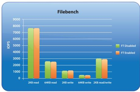
FT traffic 2K read: 155 Mbits/sec 2K write: 3.6 Mbits/sec 64K read: 1400 Mbits/sec 64K write: 1.96 Mbits/sec 2K read/write: 34 Mbits/sec
