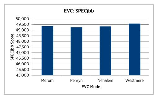
Figure 4. Scores from SPECjbb runs with different EVC modes
