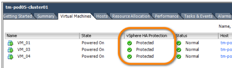
Figure 4. vSphere HA Protection States of the Virtual Machines
