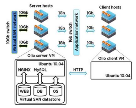
Figure 1. Host connectivity and component configuration
