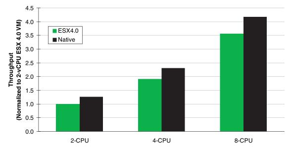
As the ratios in Figure 2 show, ESX 4.0 scales extremely well; for each doubling of processors, throughput increases by about 90%.
