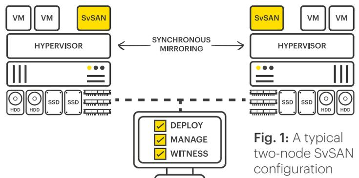
Fig. 1: A typical two-node SvSAN configuration
