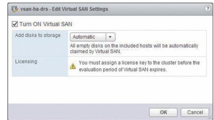
**VMware Virtual SAN is built within vSphere 5.5, by checking the related box you can activate it if you have the proper software license.**
