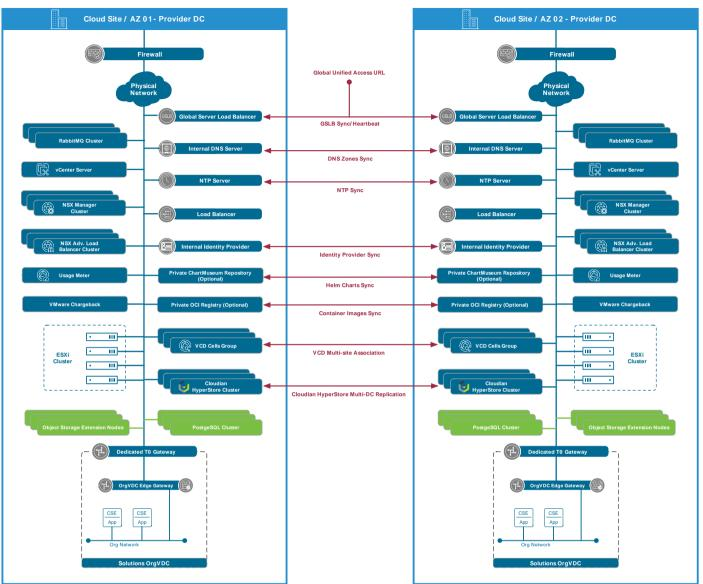
Figure 8: OSE Deployment in Multi-Site / Multi-AZ Configuration
