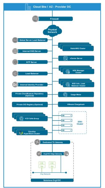
Figure 3: CSE Deployment in each AZ (new components marked in green)
