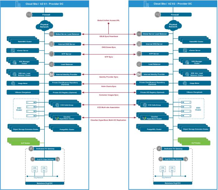
Figure 11: ALP Deployment in Multi-Site / Multi-AZ Configuration
