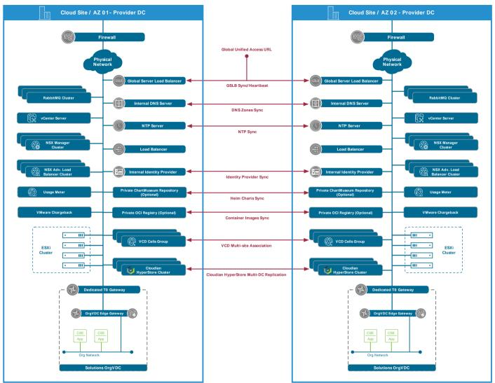
Figure 5: CSE Deployment in Multi-Site / Multi-AZ Configuration
