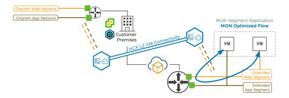
Mobility Optimized Networking can be configured to allow migrated virtual machines to reach S3 storage endpoints.
