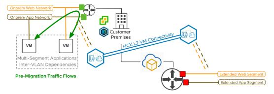
Without MON, HCX Network Extension expands the on-premises broadcast domain to the VMC SDDC while the first hop routing function remains at the source. The network tromboning effect is introduced observed when virtual machines connected to different extended segments communicate.
