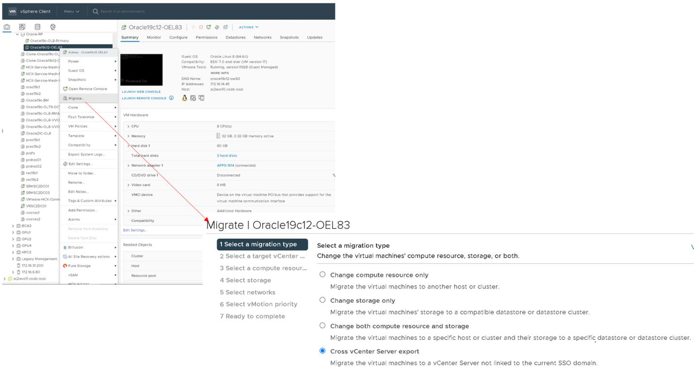
FIGURE 61. Cross vCenter vMotion for VM Oracle19c12-OEL83
