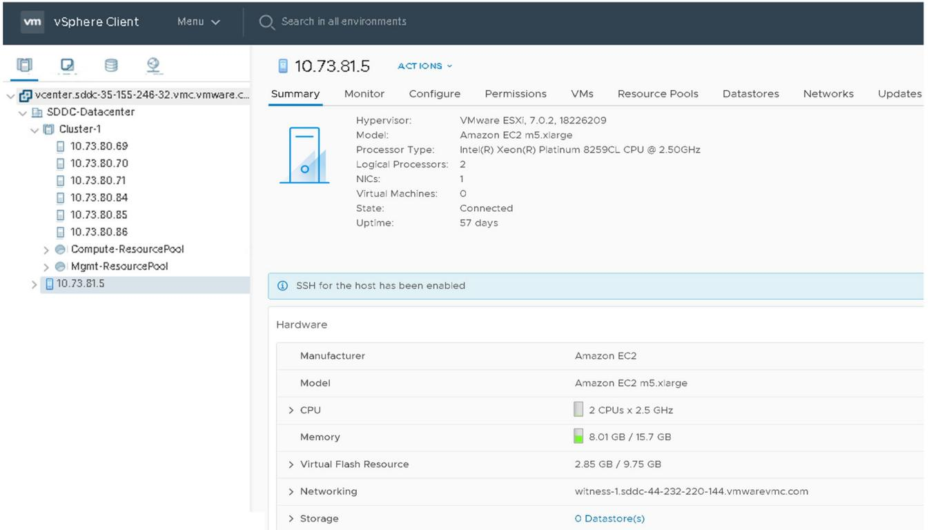
FIGURE 21. Witness in Stretched Clusters for VMware Cloud on AWS
