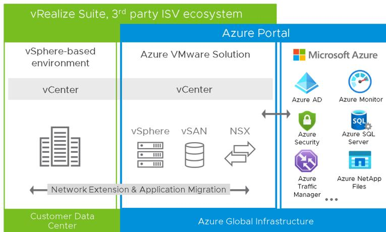
FIGURE 8. Azure VMware Solution
