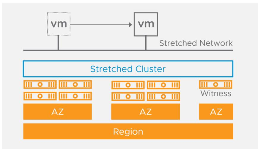
FIGURE 5. Stretched Clusters for VMware Cloud on AWS
