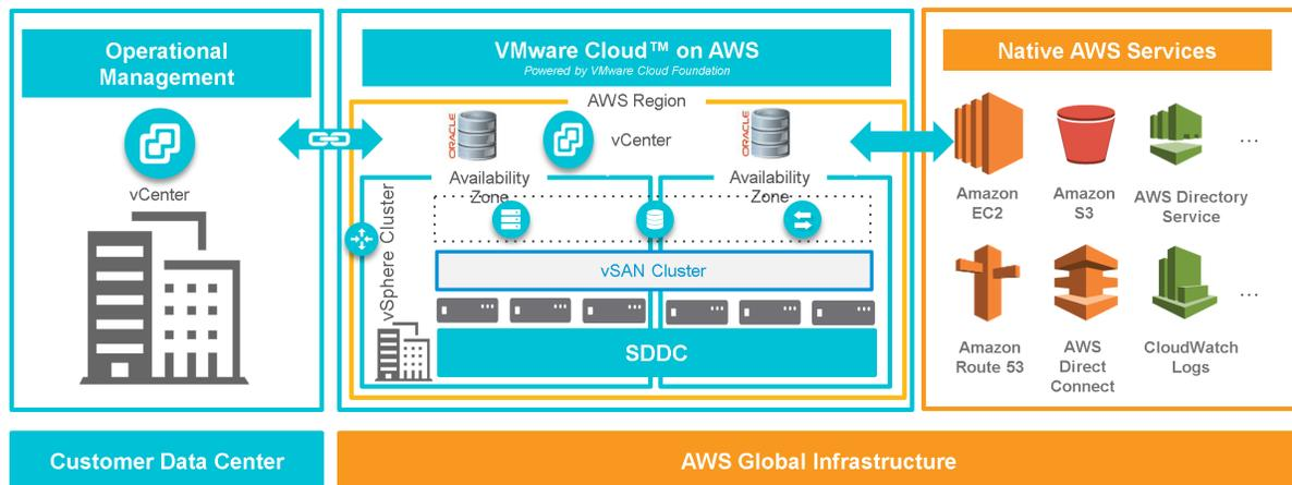
FIGURE 12. Stretched Clusters for VMware Cloud on AWS
