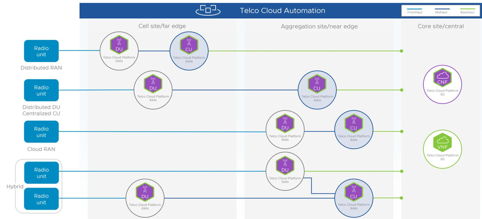
Figure 1: Enabling flexible 5G RAN deployment with a consistent horizontal platform
