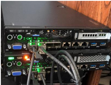
Lenovo ThinkSystem SE350 2-node Edge cluster with 10GbE SFP+ interlink cables
