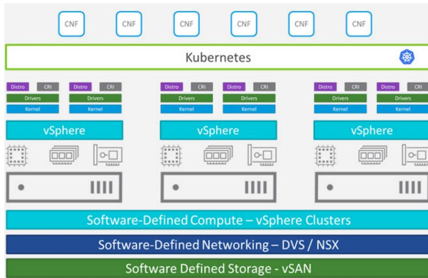
The architecture of Kubernetes on vSphere in VMware Telco Cloud Platform. The architecture puts in place horizontal software-defined infrastructure for compute, networking, and (optionally) storage.
