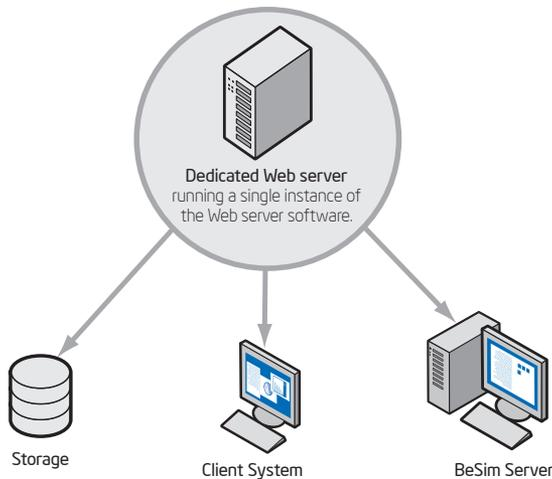
**Figure 1. Test Configuration for the Dedicated Web Server.** Performance was measured for a two-socket Intel® Xeon® processor 3.60 GHz-based server running a single instance of Microsoft IIS.\*
