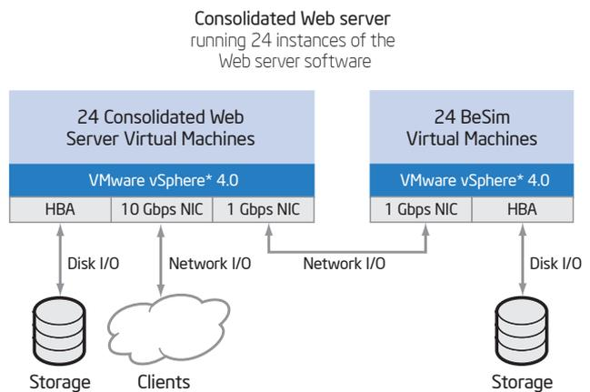
**Figure 2. Test Configuration for the Consolidated Web Server.** Performance was measured for a single Intel® Xeon® processor X7560 series-based server running VMware ESX\* Server 4.0 and twenty-four instances of Microsoft IIS.\*
