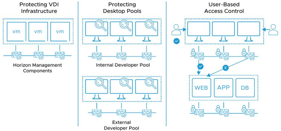
**FIGURE 1:** Distributed Firewall protects VDI, virtual desktops and applications
