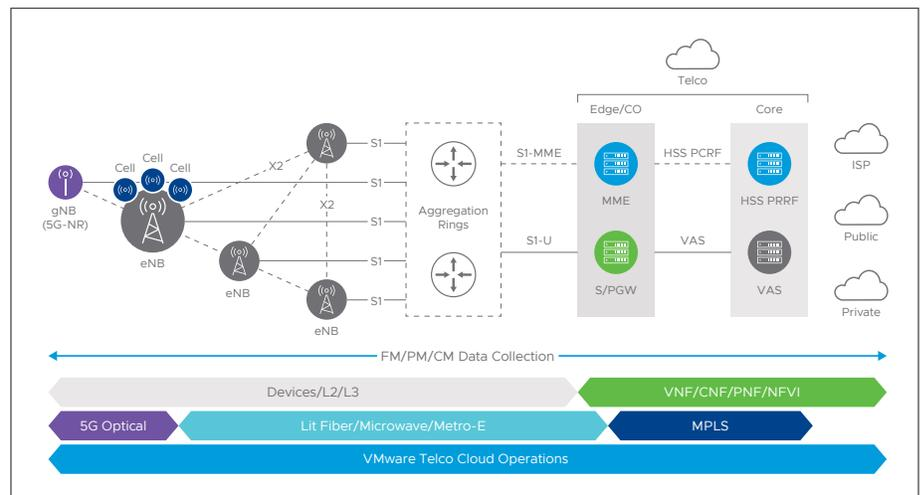
FIGURE 1: VMware Telco Cloud Operations Provides E2E Automated Assurance in a 5G Non-Stand-Alone (NSA) Environment
