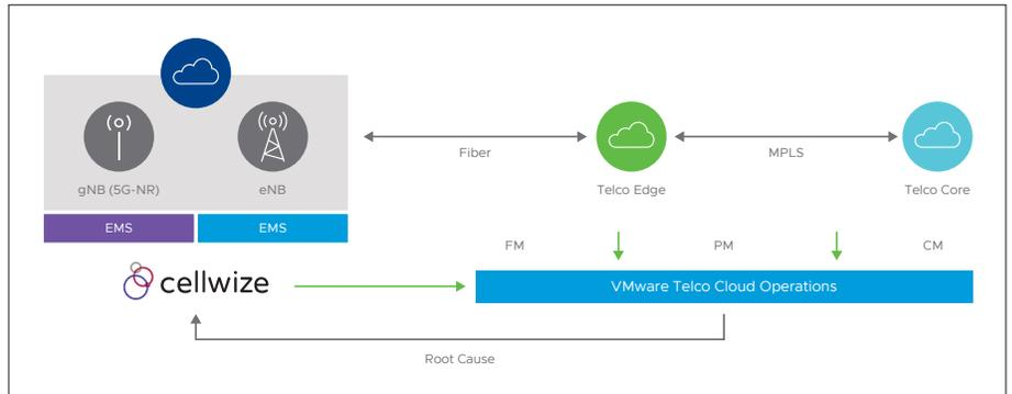
FIGURE 2: Prescriptive Root Cause Analysis in Both the RAN and IP Core Networks
