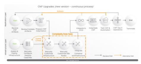
FIGURE 3: A view of a CNF upgrade before the use of Dynamic Infrastructure Policies. Without Dynamic Infrastructure Policies, the customizations of Kubernetes nodes and virtual infrastructure are highly complex tasks requiring expertise in customizing applications, Kubernetes nodes, and other infrastructure, such as the virtual machines. These tasks usually require professional services and can lead to rollbacks and misconfigurations.
