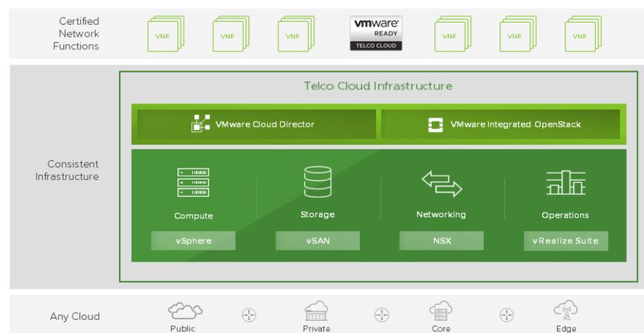
FIGURE 1: The architecture of VMware Telco Cloud Infrastructure, which provides consistent infrastructure to simplify, scale, and protect the operation of multi-vendor network functions.
