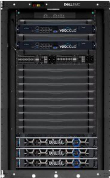
FIGURE 2. VMware Cloud on Dell EMC infrastructure rack
