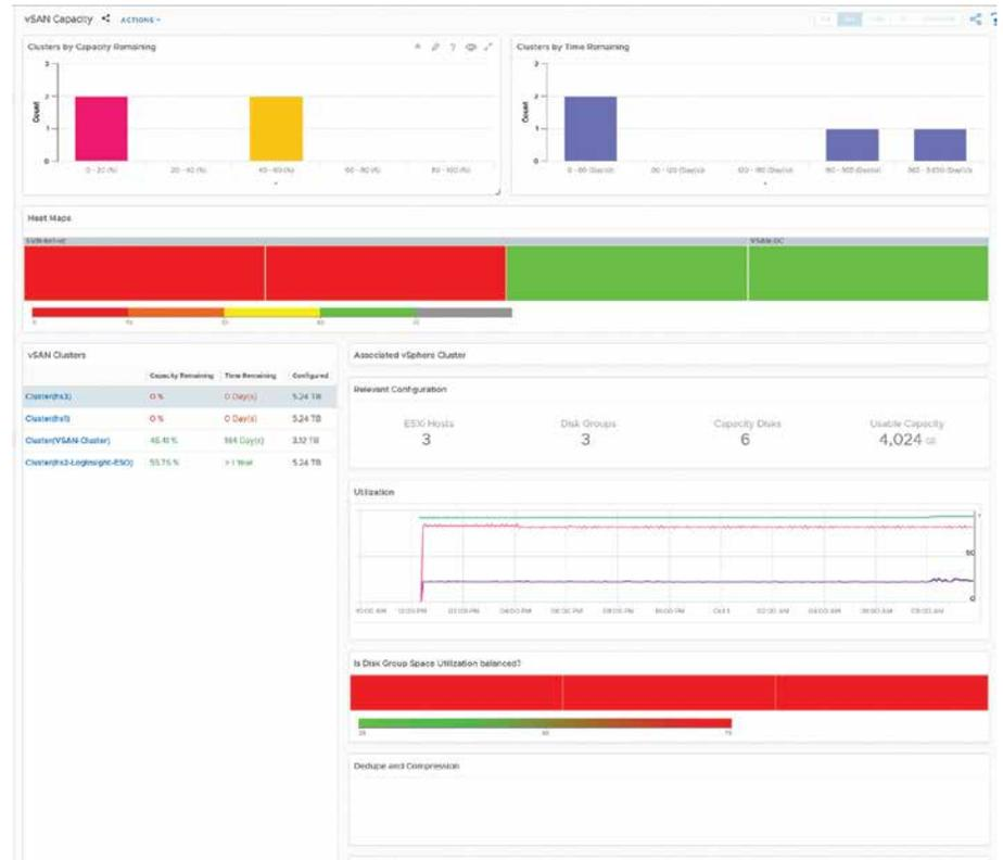
FIGURE 4: The vSAN Capacity dashboard.
