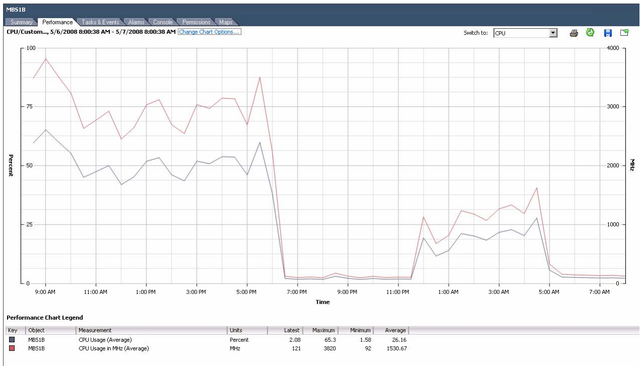
Figure A-3. VirtualCenter CPU performance data for one of the mailbox virtual machines
