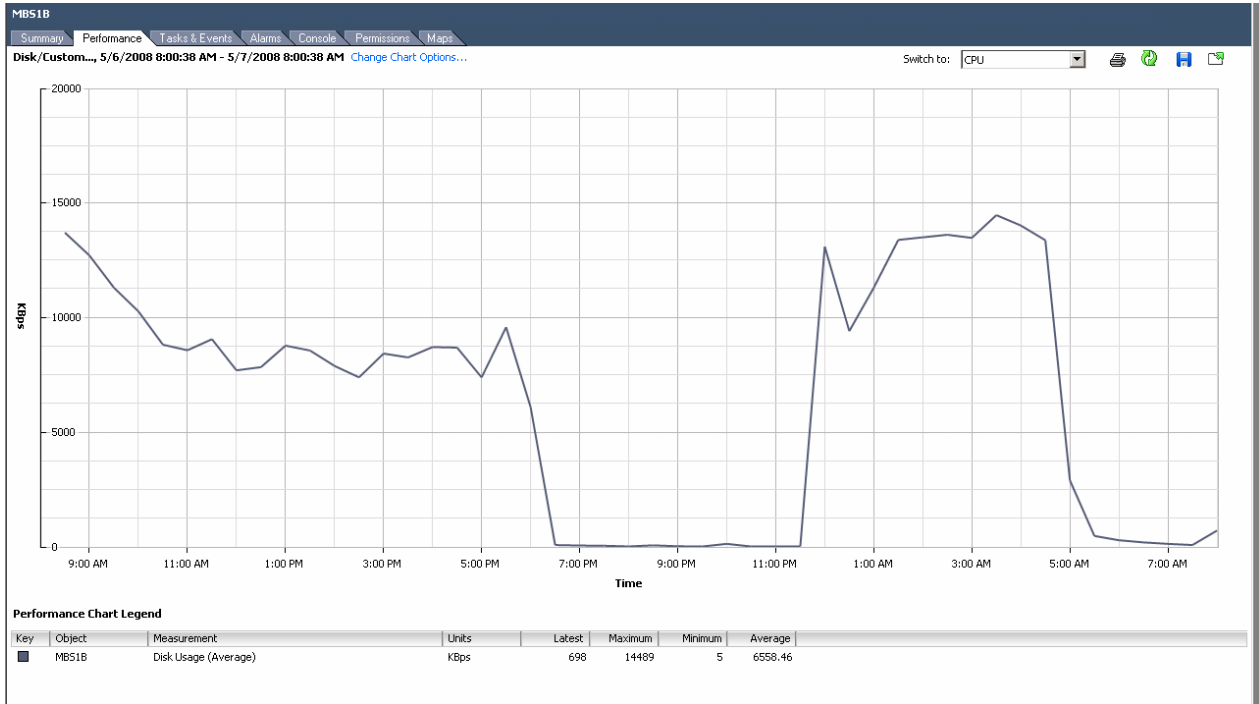
Figure A-7. VirtualCenter disk performance data for one of the Mailbox Virtual Machines
