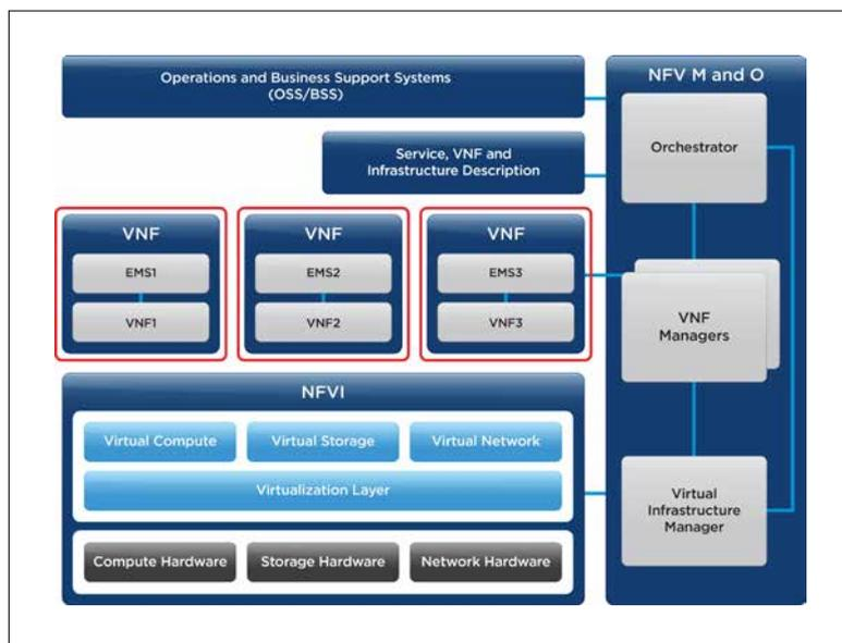
Figure 3: Scenario 2 - A Horizontal Virtualization Blueprint allows on-boarding of multi-vendor services
