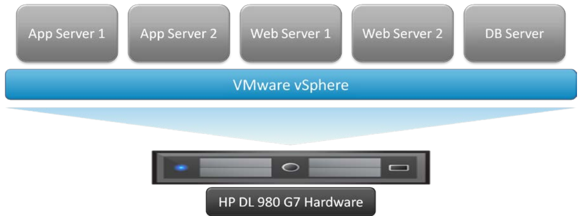
Figure 5: Test Bed for Two APX Firm on ESX Host
