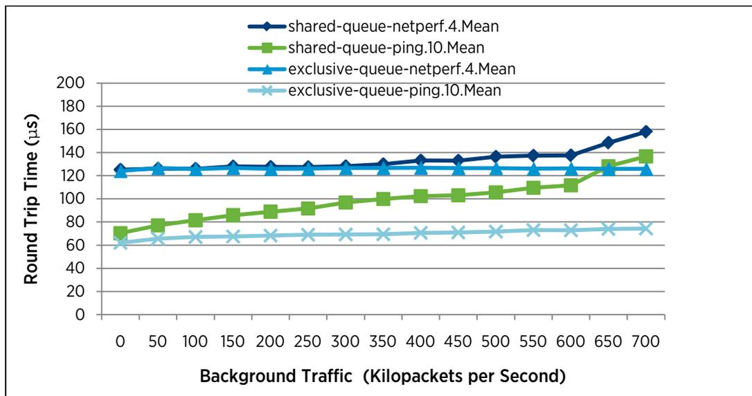
Figure 9. Round-trip time under Rx bandwidth contention
