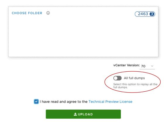
Figure 12. In this screenshot, you would need to enable **All full dumps** (as marked in red) before uploading your dump file. You would click the toggle to enable it.
