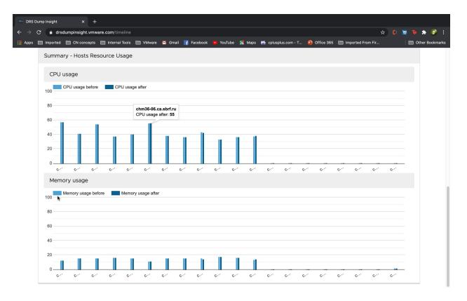
Figure 6. For every host in the cluster, resource usage is shown before and after the given DRS run.
