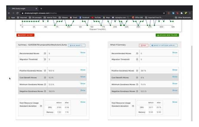
Figure 8. After the what-if analysis completes, you can see a side-by-side comparision of the details of the run with and without the applied what-if options.
