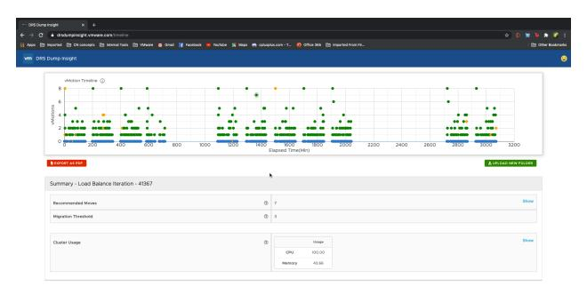
Figure 10. DRS Dump Insight for DRS 2.0 (vSphere 7.0 and 7.0 U1) displays the vMotion timeline when dump files are uploaded for analysis.
