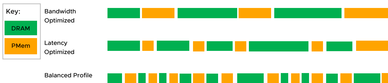
Figure 1. This shows the profiles of DRAM and Intel Optane PMem traffic. DRAM is green; PMem is orange.
