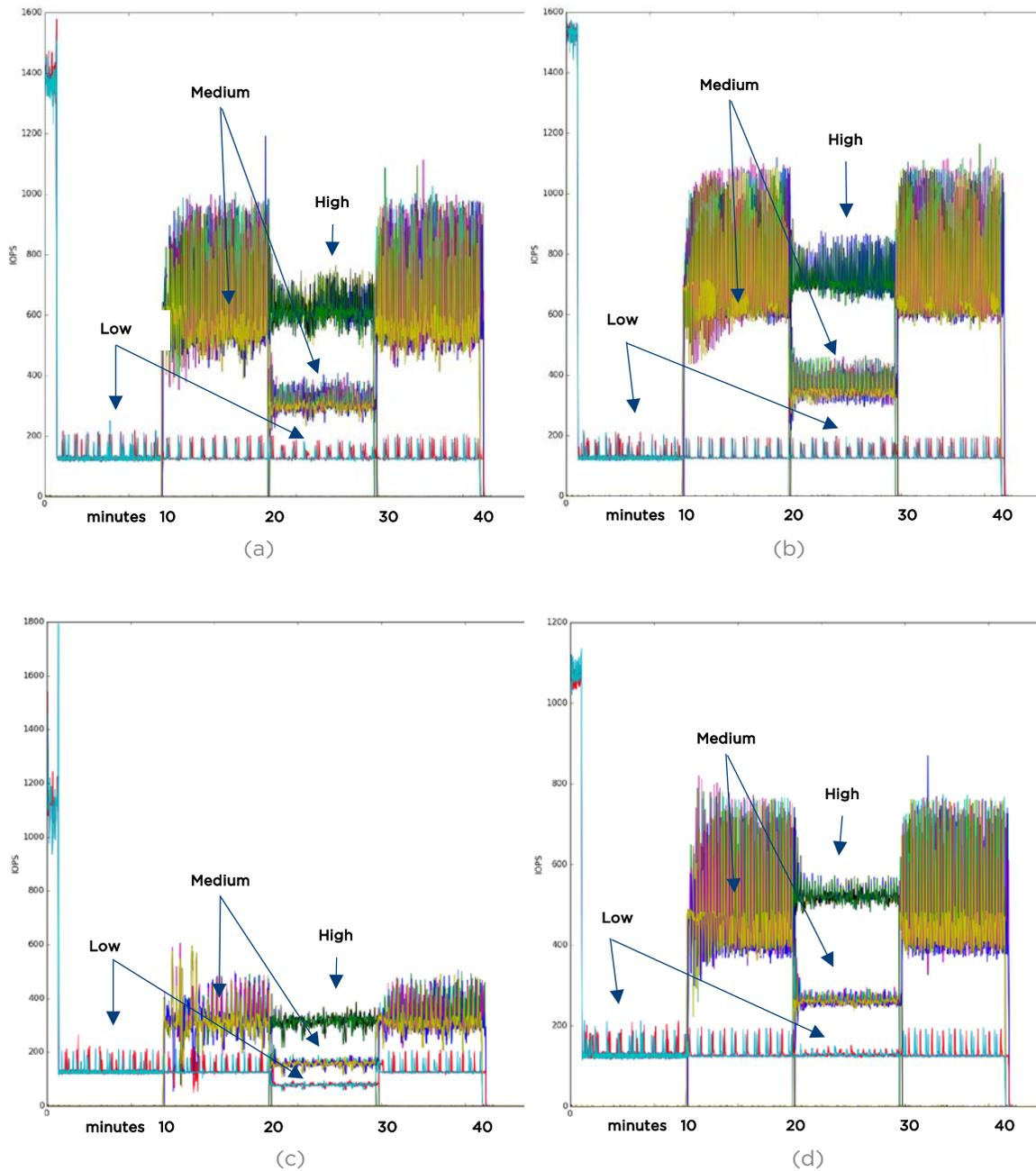
Figure 6. Performance impact of using SIOC in datacenter. (a) sequential write, (b) sequential read, (c) random write and (d) random read
