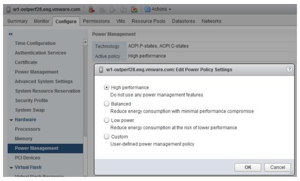
Figure 5. Power Policy Settings in the vSphere Web Client
