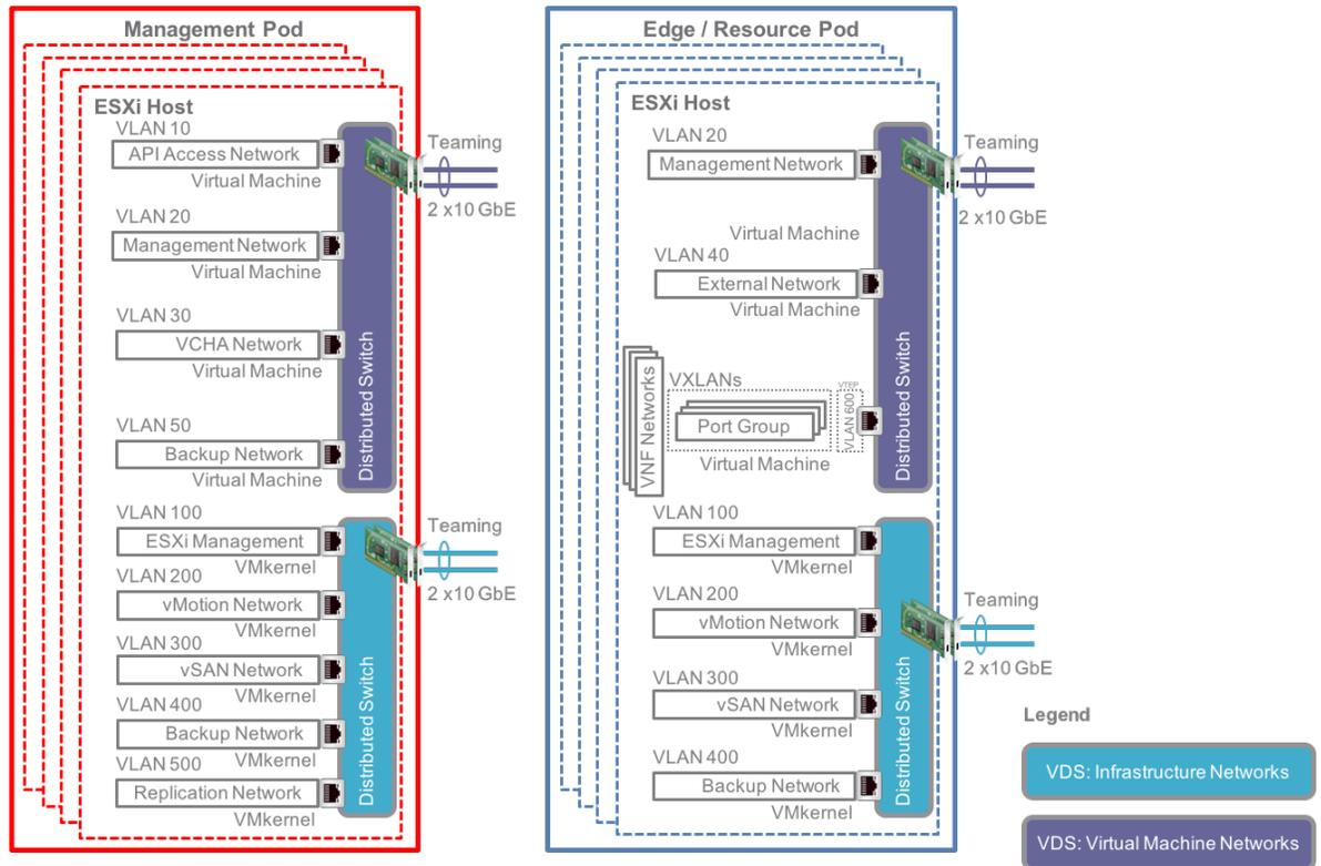
Figure 10: Distributed Virtual Switch Two-pod design
