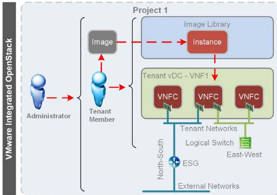
Figure 26: VMware Integrated OpenStack VNF Onboarding
