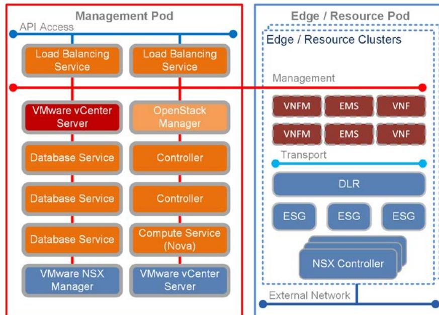
Figure 11: VMware Integrated OpenStack Two-pod design
