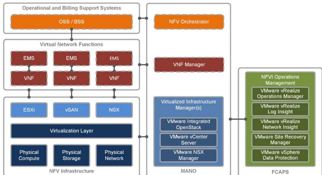
Figure 2: Mapping Functional Elements to the ETSI NFV Reference Model
