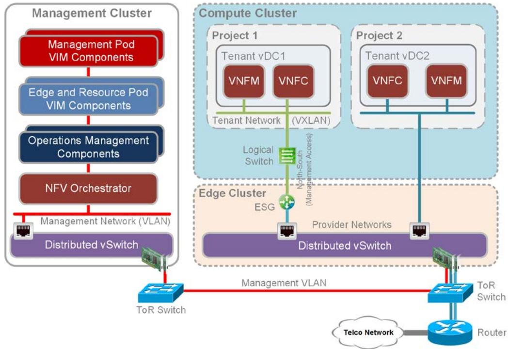
Figure 27: VNF Networking with VLAN Backed External Network
