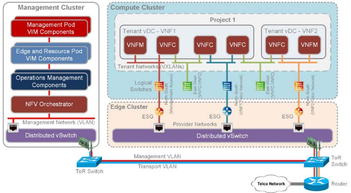
Figure 28: VNF Networking in Three-Pod Design
