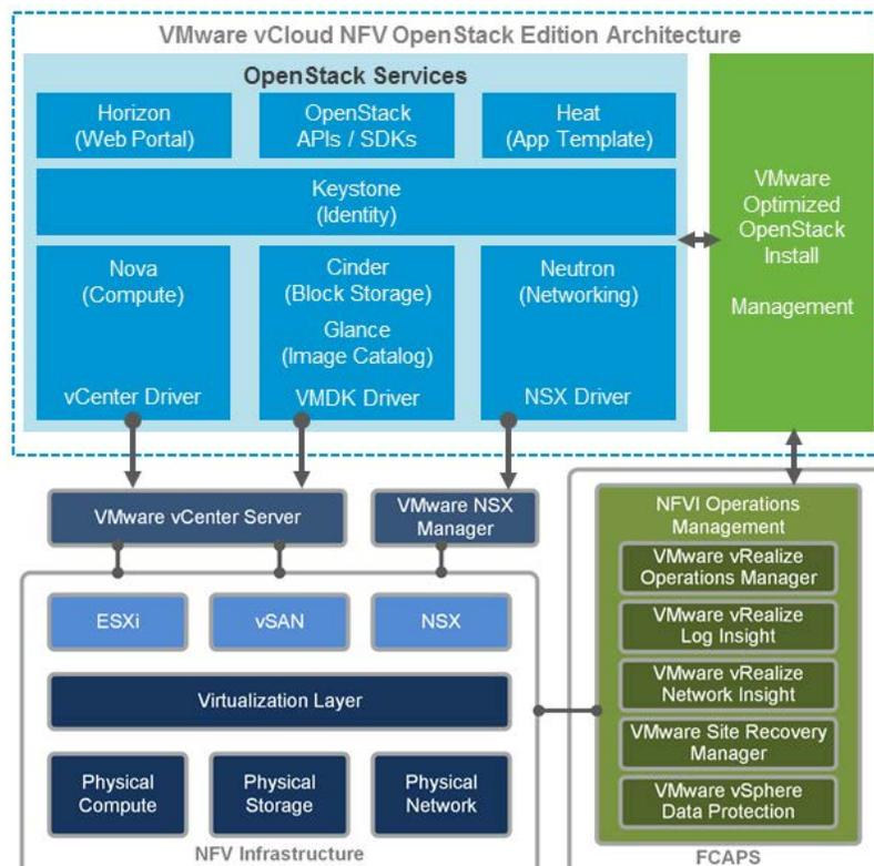
Figure 5: VMware vCloud NFV Integrated OpenStack Architecture
