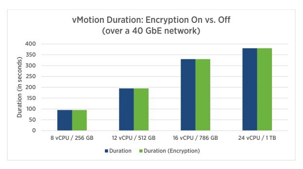
Figure 4. Encryption does not affect vMotion performance over a 40 GbE network
