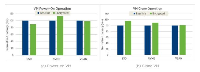
Figure 8. Performance of powering on VMs and cloning VMs on different storage devices (lower is better)
