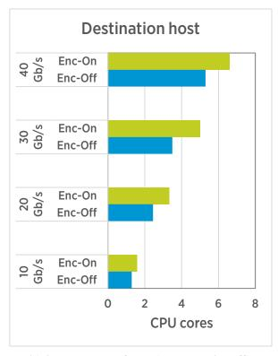
Figure 5. vMotion requires more CPU cores to manage higher amounts of vMotion network traffic
