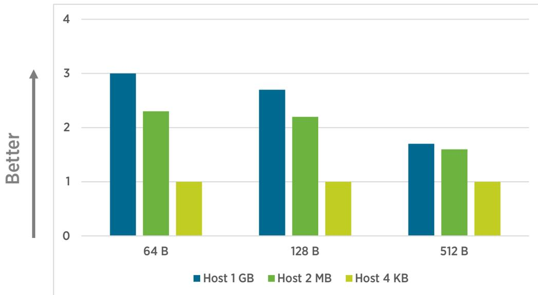
Figure 1. The host with an access size of 1 GB performed 26% better than the host with an access size of 2 MB
