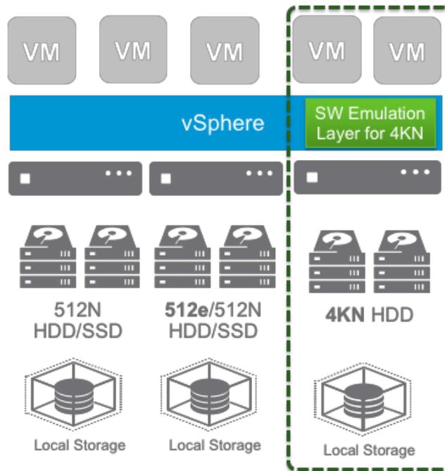
Figure 5. vSphere 6.7 includes software emulation for 4Kn drives
