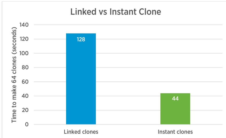
Figure 4. Instant clone performance (fully clone and boot 64 clones) – lower is better
