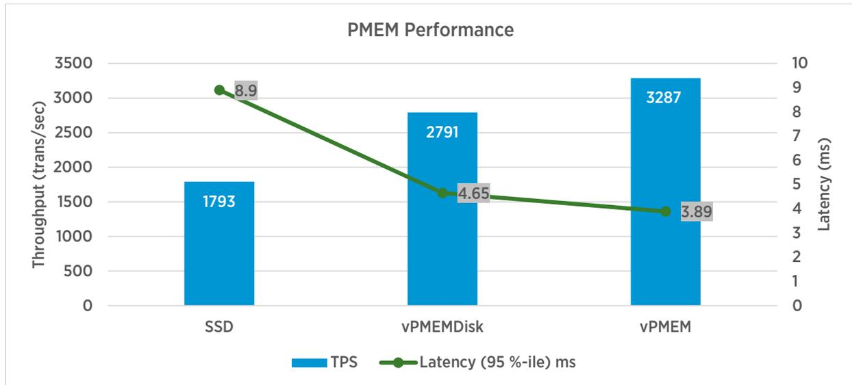
Figure 2. Virtual PMEM can improve performance by up to 1.8x better throughput and 2.3x better latency over standard SSD technology
