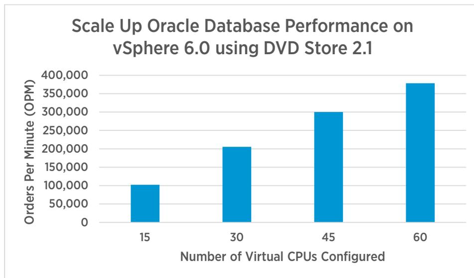
Figure 2. Scale-up test results up to 60 vCPUs
