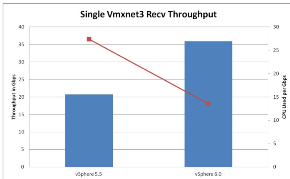
**Figure 5. Comparison of throughput and CPU usage for 40GbE with VMXNET3 on vSphere 5.5 and 6.0**
