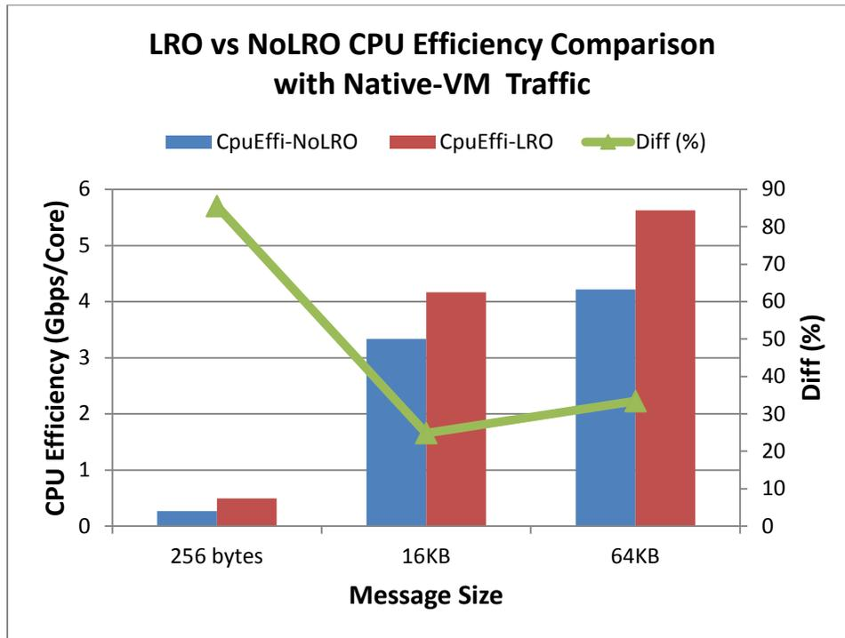
Figure 4. CPU efficiency comparison with and without LRO with Native-VM traffic
