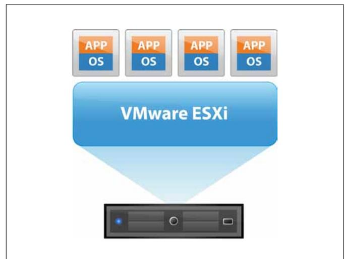
Figure 1. Server Consolidation with VMware vSphere
