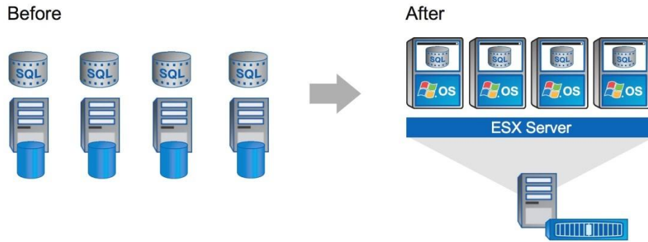
Figure 3) Consolidate multiple physical instances of Microsoft SQL Server onto a single VMware server and reduce both hardware and license costs.
