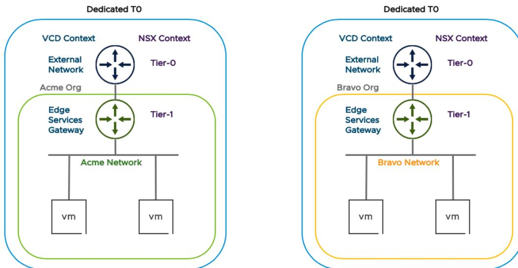
Using a Dedicated T0 is permissible when using VCD 10.1 or greater. In this model, the provider will create a T0 that is exposed as an External Network within VCD. However, the provider will select the option “Dedicate External Network” during the Edge Service Gateway wizard creation. Once this option is selected, the tenant has a complete T0 and T1 dedicated to their oVDC environment.
