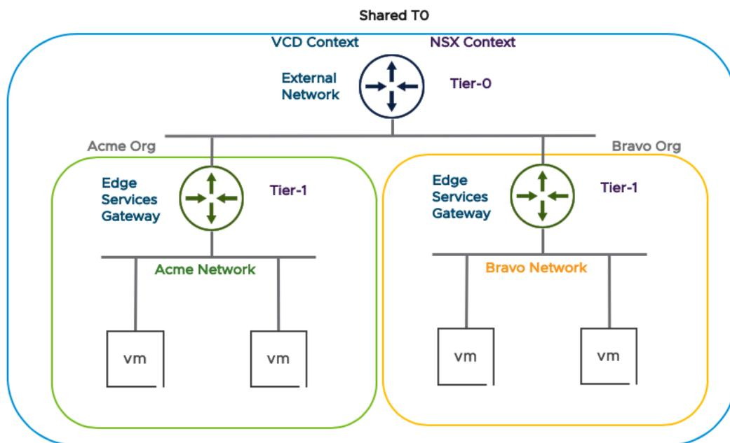
Within a Shared T0, the provider creates a T0 which is exposed as an External Network to VCD. Upon completion, the provider can create orgVDC Edges that are instantiated as T1's. As Figure 21 depicts, the newly-created Edge Service Gateway, or T1, is automatically connected to the northbound T0.
