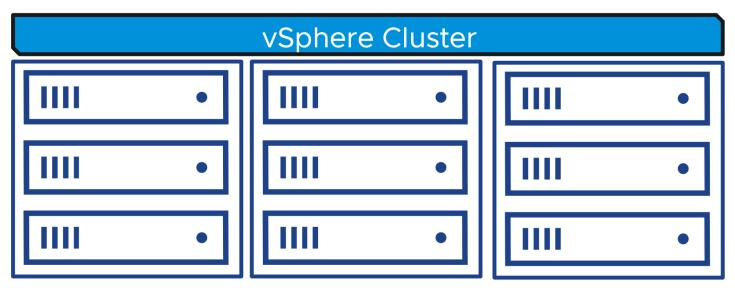
vSphere HA feature such as VM and Application monitoring supports VMware Tools heartbeat monitoring for vCenter Server and VM Component Protection (VMCP) helps protect against datastore accessibility issues and can restart vCenter Server on another host if the current host has issues accessing the datastore.
