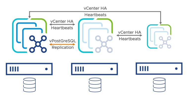
During a vCenter HA failover event, the vCenter Sever services must start on the new active node. The failover is not instantaneous and there will be some down-time until the services have completely started. vCenter HA heartbeat monitoring is also available via the the vmware-vcha service to monitor the liveliness of the three vCenter HA nodes from the perspective of the vCenter HA cluster.
