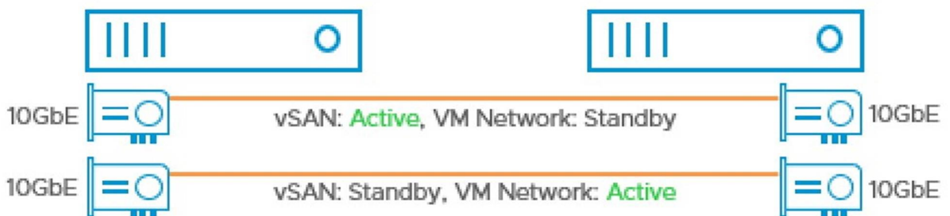
Figure 8. Networking Design of FTT=1 Configuration with two 10 GbE NICs
