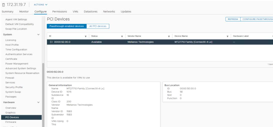
**Figure 32. Mellanox Network Adapter is Configured to Passthrough**
