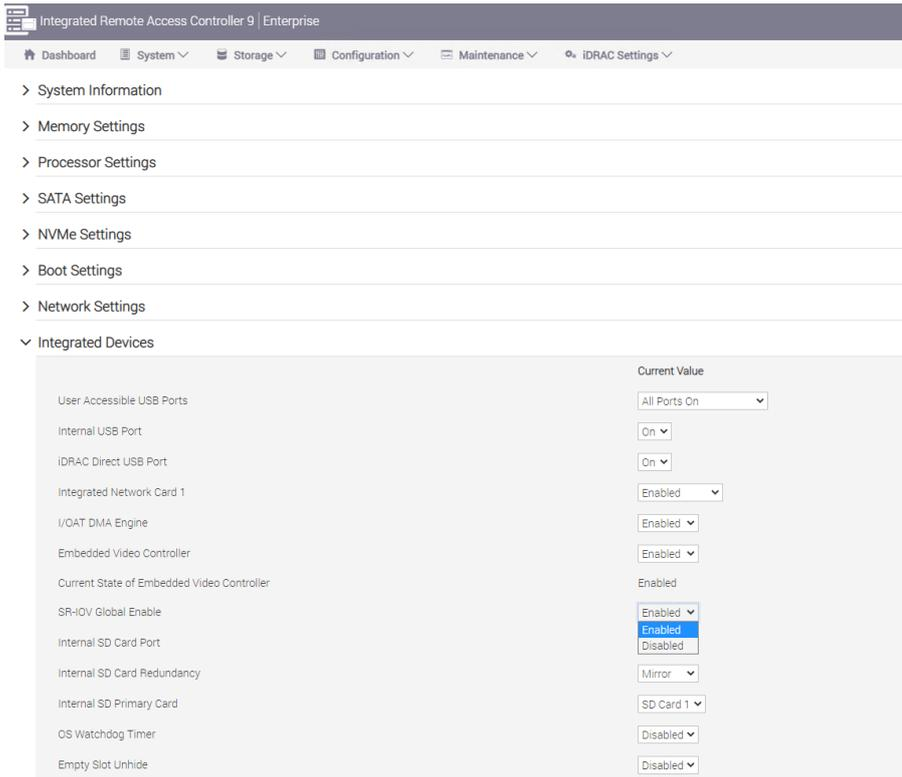
Figure 5. Enable Global SR-IOV in iDRAC
