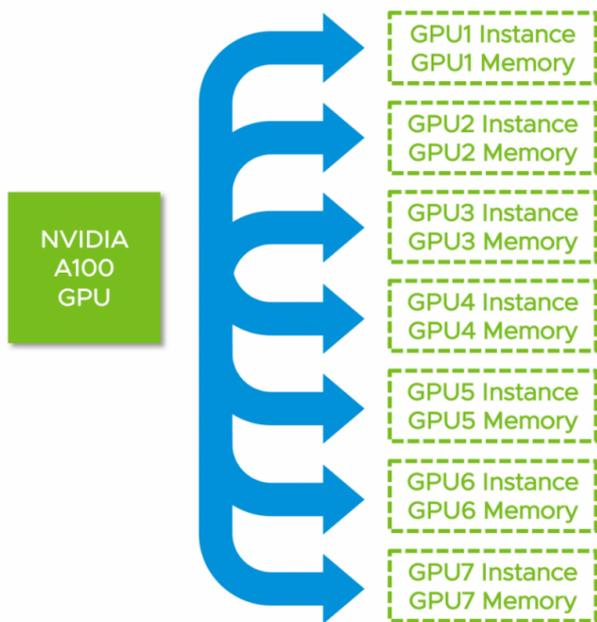
**Figure 2. NVIDIA A100 Multi-Instance GPU**
