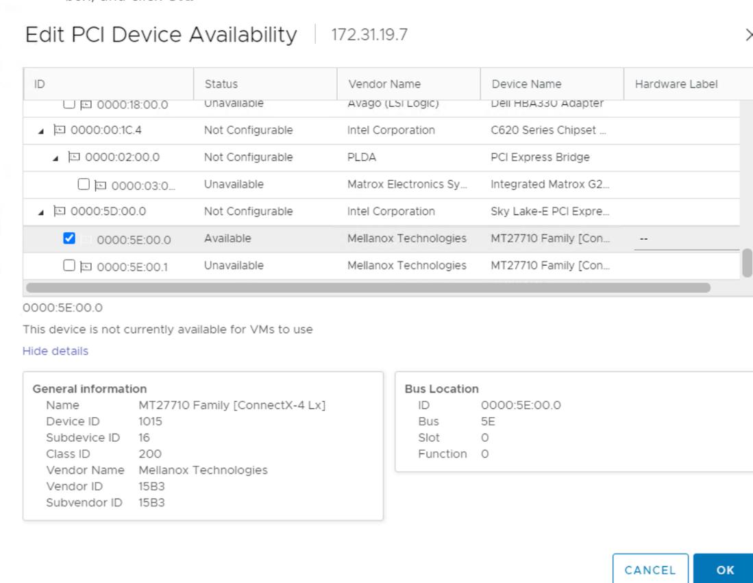
**Figure 31. Select Mellanox Network Adapter to Passthrough**
