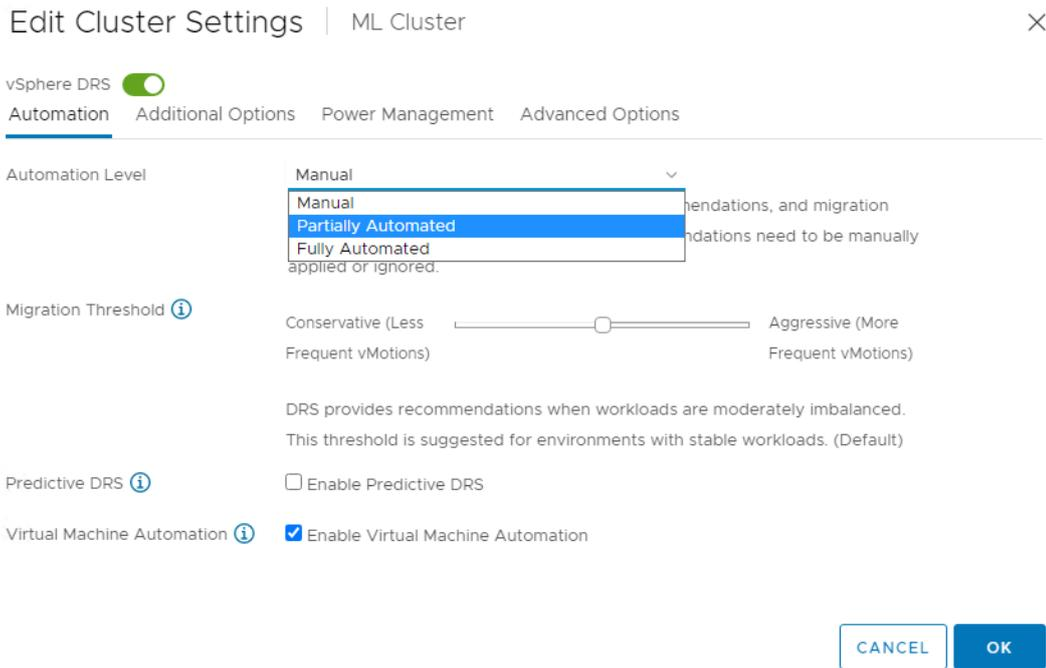
**Figure 6. Configure DRS Automation Level to Manual or Partially Automated**
