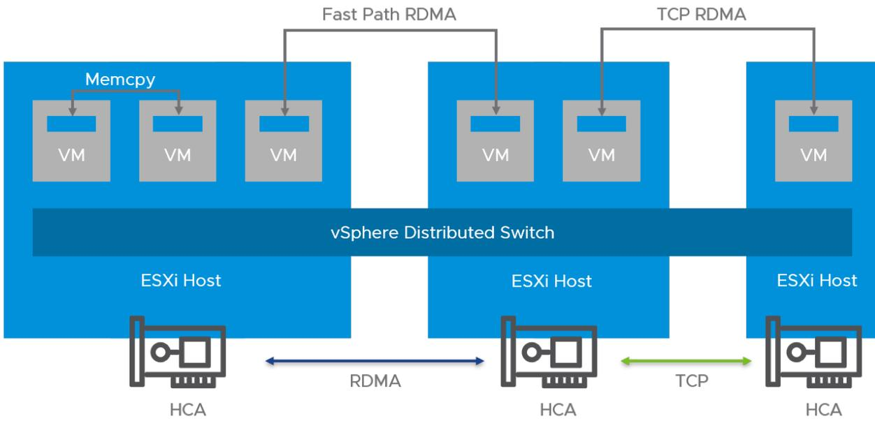
Figure 3. Paravirtual RDMA Architecture
