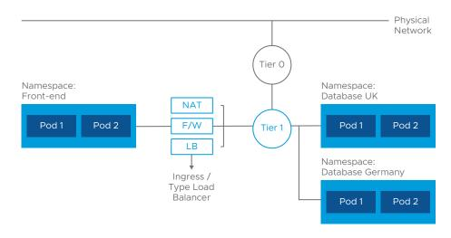
FIGURE 8: NSX provides full-stack networking and security services to vSphere with Kubernetes.
