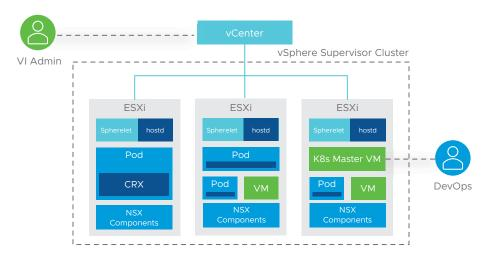
FIGURE 3: VMware NSX is designed into vSphere with Kubernetes. NSX components include the NSX Container Plug-in, vSphere Distributed Switch™ and NSX Agent.
