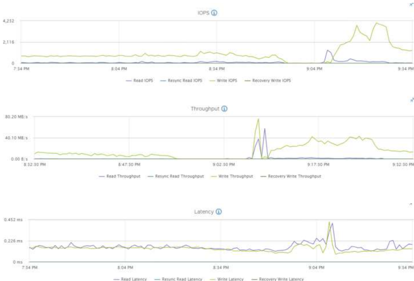
Figure 10. vSAN Backend Performance Results during Provisioning Instant Clone Desktops
