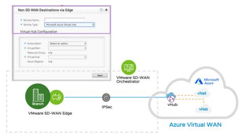
FIGURE 1: VMware SD-WAN Edge to Azure Virtual WAN Hub
