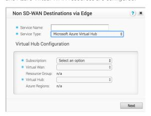
$\hbox{FIGURE 3: Configuration step in VMware SD-WAN Orchestrator GUI for direct connect from VMware SD-WAN Edge } \\$
