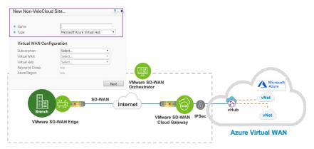
FIGURE 2: VMware SD-WAN Edge to VMware SD-WAN Gateway to Azure Virtual WAN Hub
