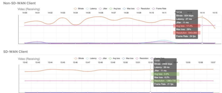
Figure 3: VMware SD-WAN: loss mitigation for better resolution for Zoom video communications
