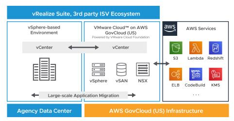
Figure 1: VMware Cloud on AWS brings VMware's enterprise-class Software-Defined Data Center software to the AWS Cloud and enables customers to run production applications across VMware vSphere-based private, public and hybrid cloud environments, with optimized access to AWS services.
